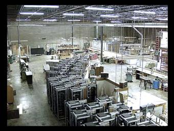
Raceways are delivered with all specified components factory installed. They are set in place, ganged & turned over for power data termination the same day; providing substantial savings in the customer's time & money.
