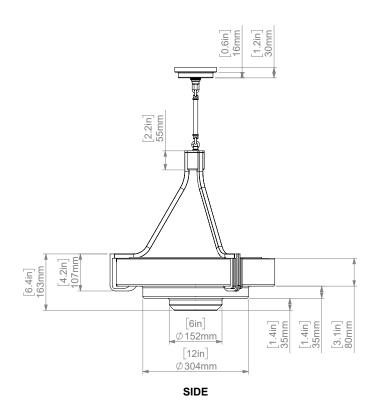
Due to the hand-crafted nature of some products, stated dimensions may have a tolerance of  $\pm \frac{1}{4}$ %mm. If tighter tolerances are required for a specific installation, please state on your enquiry
